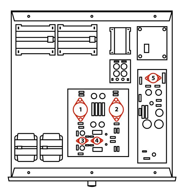
VALVE 1; 300B VALVE 2; 300B VALVE 3; 5687 VALVE 4; ECC82
